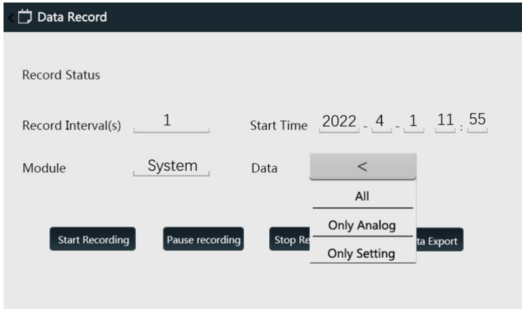
Figure A- 6 Sinexcel 7-inch HMI Data Record Setting
