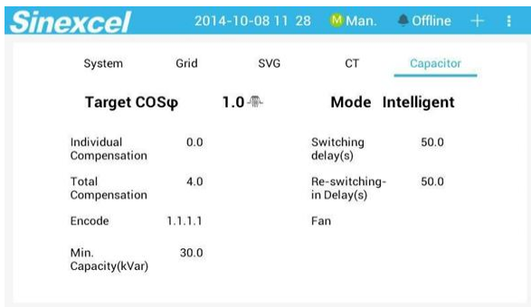
Figure A- 62 Capacitor settings information
