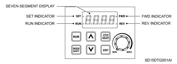
The LED indicators turn on or flicker, showing the current operation status of the drive. The following table lists the names and functions of the operating keys on the display:
