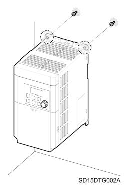
Mount the drive on the wall or inside the panel using the top two bolts and then fully tighten the mounting bolts. Ensure that the drive is placed flat on the mounting surface and that the surface can securely support the weight of the drive. Use the following image as a guide.
