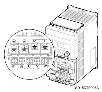
The motor chassis ground must be connected to the drive. In other words, connect the motor's ground conductor to the PE protection terminal of the drive and not to the installation's ground. It is recommended that the section of the motor ground conductor (PE) has at least the same cross section as the motor power cables sections (U, V, W). Additionally, it must be installed following the recommendations indicated in sections <u>Power connection and wiring</u>.
