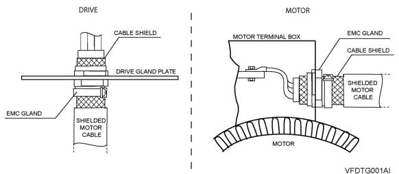
It is recommended to use shielded cable for control signals and to follow recommendations included in section <u>Wiring recommendations</u>.
