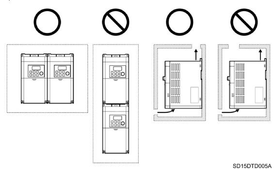
If multiple equiment of different sizes are installed, it is necessary to leave sufficient clearance to meet the clearance specifications of the largest drive.
