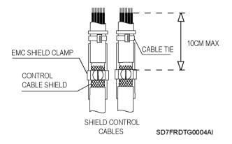
Cable shields for digital signal must be grounded at both ends of the cable. It is recommended to use independent shielded cables for digital and analogue signals. When using multiple analogue signals, do not use common return for them. If using analogue signals, a low interference is experienced (hum loops), disconnect the shield grounding from one of the ends. Refer to <u>Recommended cable section</u> for cable specifications and recommended adjustment.
