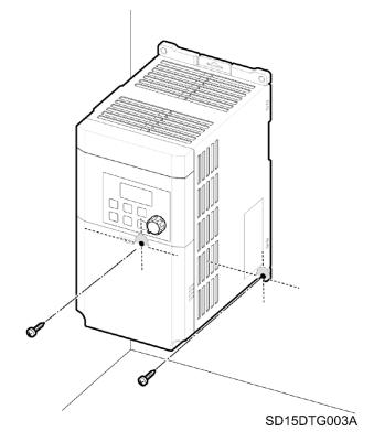
**Note**: The quantity and dimensions of the mounting brackets vary based on frame size. Please refer to section <u>Dimensions</u> to find the information that corresponds to your model.
